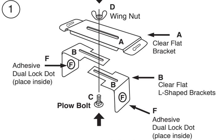
Assemble brackets, leaving the **Wing Nut (PART D)** loosely threaded onto **Plow Bolt (PART C)**
