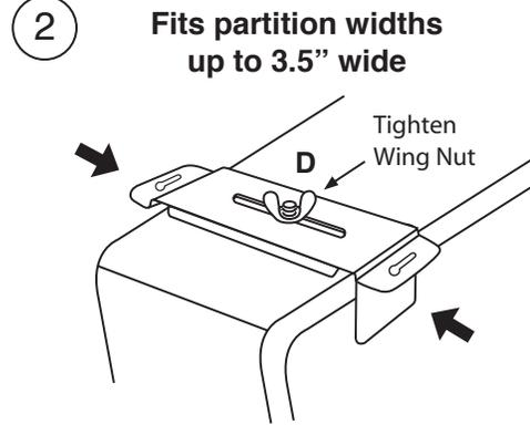
Position brackets onto top of partition, adjusting for width and a tight fit. **Tighten Wing Nut (PART D)**
