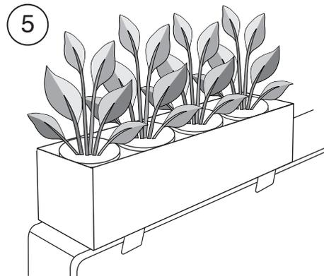
Load your planter container with plants and top dressing as desired. Re-align screws from bottom of planter to pre-drilled slots on brackets and slide into place.
