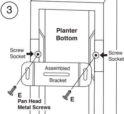
Remove assembled bracket from partition. Insert **Pan Head Screws (Part E)** into screw sockets on bottom of planter. Align assembled bracket. (Allow for space for bracket to be able to slide)
