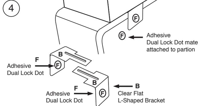
Attach one Transparent **Dual-Lock Adhesive Dot (PART F)** to inside of each **L-Shaped Bracket (PART B)** and its corresponding mate to the partition wall so they will match up (repeat for remaining bracket parts)
